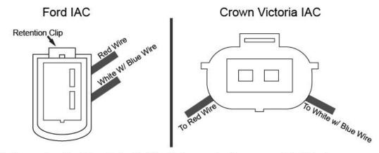
Cut these wires 1 inch from the back of the Ford connector. Then connect Red Wire to new IAC pigtail Red Wire on the Crown Victoria using included pink heat shrink butt connectors. Repeat step for the White with Blue Stripe Wire.
