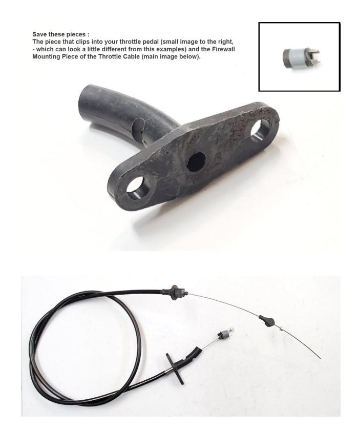
You can now assemble your new throttle cable with all the components. It helps to put your components all together and through before you attach the firewall piece onto the cable housing. It is a pain to, but if you leave the un-crimped end towards the throttle body it will make
