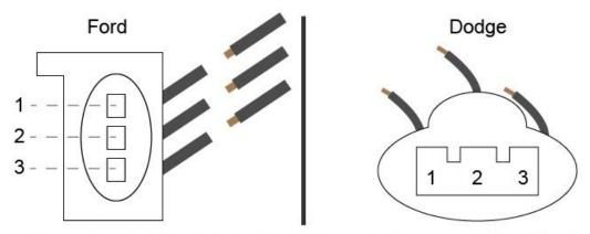
Cut these wires 1 inch from the back of the Ford connector. Then connect Wire #1 from the harness to new TPS pigtail wire #1 on the Dodge using included pink heat shrink butt connectors. Repeat step for wires #2 & #3. Do not concern yourself with the colors of the wires, only the number sequence.
