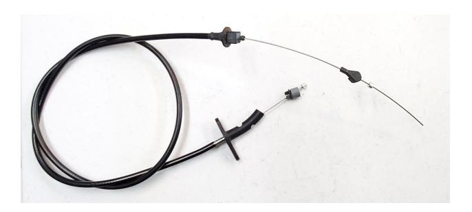
You can now assemble your new throttle cable with all the components. It helps to put your components all together and through before you attach the firewall piece onto the cable
